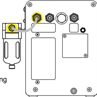
Cut the black hose 139mm (5 1/2"). Connect one end to the **air input quick connect fitting** on the back of the machine and the other end to the straight **quick connect fitting**.
