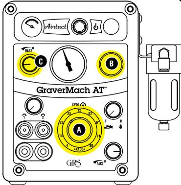
Hold the handpiece you have selected to use vertically, tool holder end up, next to your ear. Without depressing the foot throttle or palm control, **SLOWLY** increase the air pressure until the handpiece begins to buzz. Continue to increase the air pressure until the handpiece vibrates and knocks. Slowly add air pressure until the knocking stops. This is the perfect air pressure for each handpiece. Now you are free to move the SPM (strokes per minute) dial to whatever setting desired.
